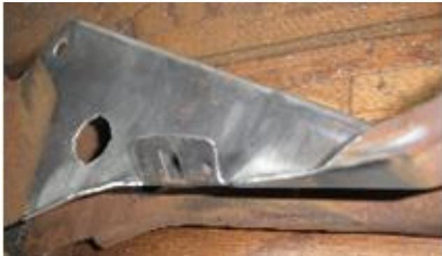
Bend the tab upward. Slot in tab needs to be as low as possible. Once folded, cut out the top of tab.
